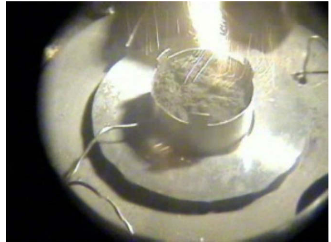
Fig. 5. First step of ignition: flash of lightning above the sample surface.
